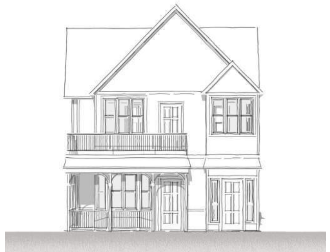
Type 2 Duplex Elevation. 2-bedroom units: Ground floor unit with second floor unit access from interior stair at side of unit.
