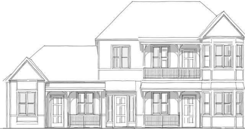
Type 1 Triplex Elevation. Two 1-bedroom units + 2-bedroom unit: 1-bedroom and 2-bedroom ground floor unit flank a central entry that provides access to an interior stair for the second floor 2-bedroom unit.
