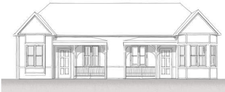
Type 1 Duplex Elevation. 1-bedroom + 2-bedroom: Side by side units with covered front porch at grade for accessibility.
