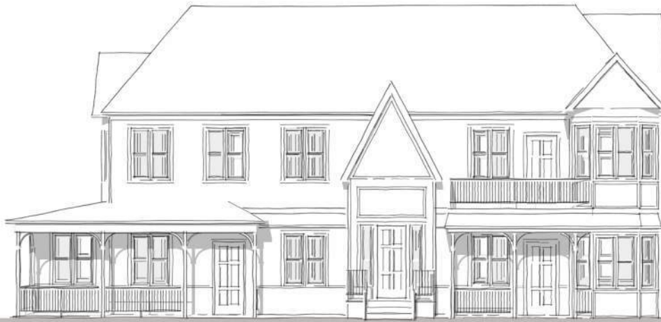
Type 1 Fourplex Elevation. Three 1-bedroom units + 3-bedroom unit: 1-bedroom ground floor units flank a central entry porch that provides access to an interior stair for the second floor 1-bedroom and 3-bedroom units.
