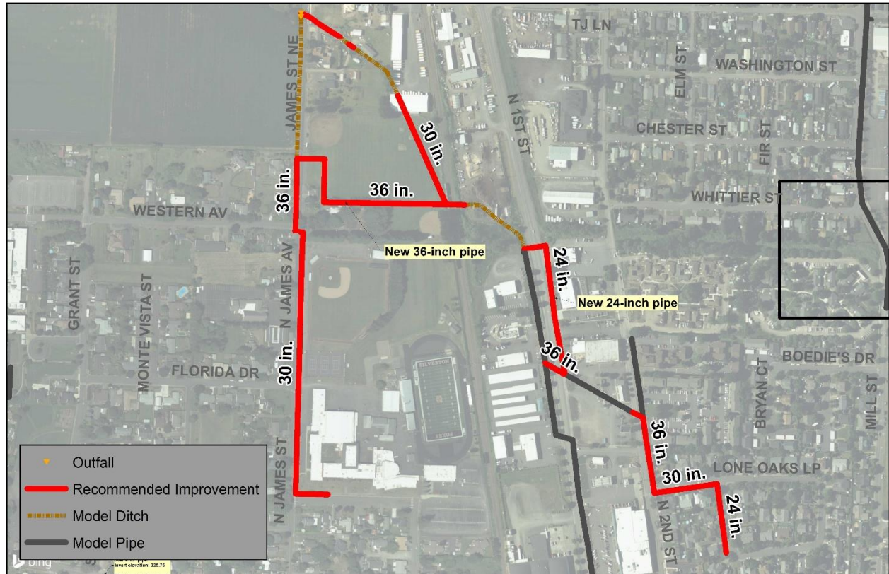
FIGURE 6-6: NORTH CENTRAL BASIN UPSIZING
