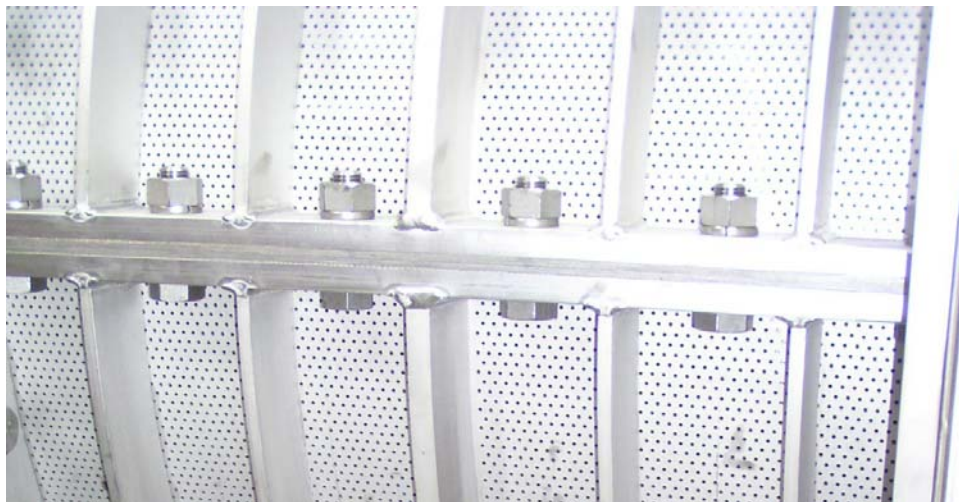
Figure 9-18: Typical Screw Press Screen
